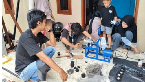
Image 3. Water Hyacinth Briquette Molding Process
