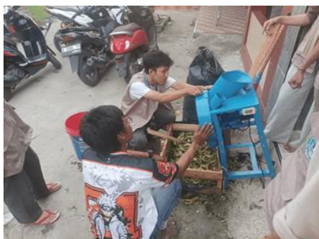
Image 1. Water Hyacinth Shredding Process
