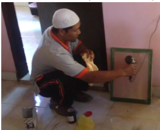
Gambar 7. Proses Pengeringan Screen Hasil Afdruck
